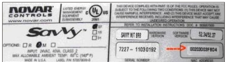
Figure 1. Sample product information label showing MAC address (lower right corner)
