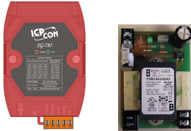
Figure 1. Novar RS-485 Biasing Module and Isolated Power Supply
