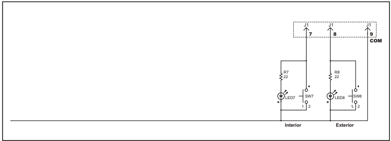
Figure 2. Wiring schematic. Resistor values are in ohms \pm 5\% .
